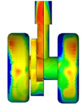
Front and rear pressure difference with design. Estimated drag reduction: 15% to 20%
